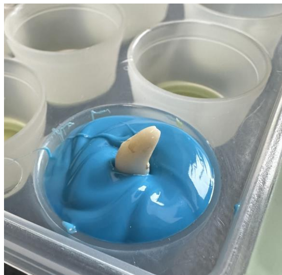
Figure 3. A tooth immersed in dental silicone while waiting for the material to polymerise.
